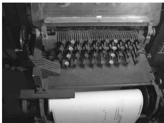
Plate 6.3 Punched paper recorder/reader of the RCA Mark II. (Photo by Thom Holmes)
