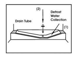
If, at any time, the defrost water does not drain from the collection channel, check that no food particles have blocked the drain tube. The drain tube can be cleared with a pipe-cleaner or Pushing the special plastic plunger provided down the drain tube (2).
