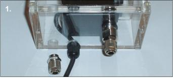
1. Screw the G1/4" fittings to the inlet and outlet making sure the o-rings are compressed. 10/8mm fittings are used in the photo but you can use any type of G1/4" fitting.
