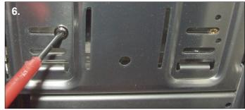
**6**. Push in the reservoir flush with the front of the PC case and use the 4 provided screws to fix it securely in place.
