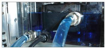
**5**. To turn on the pump connect the 4 pin power connector to a spare PSU, as the reservoir drains top up the water level. It is important that the pump does not run dry as this may cause damage. When all the air has been removed replace the filler cap and turn it clockwise to seal the reservoir.
