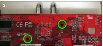
**3**. Turn the card over and line up the holes on the back of the card with the holes on the base of the GPU.
