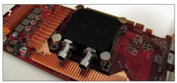
**7**. The card is now ready for use. When you first boot it is advisable to use ATItool or other software to check the core temperature. If the temperature is high you will need to remount the block.
