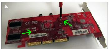
**5**. Use a philips screw driver to attach the card to the block. Do not over tighten the screws.
