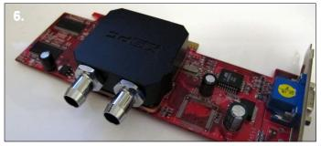
**5**. The card is now ready for use. When you first boot it is advisable to use ATItool or other software to check the core temperature. If the temperature is high you will need to remount the block.
