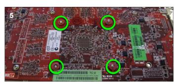
**5**. Place one hand over the GPU block and screws and turn the card over. Now place a washer over each of the screws.
