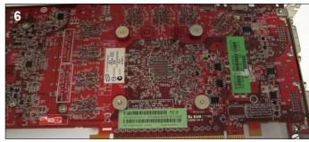
**6.** Place a nut over each of the four screws and gradually tighten each one until the correct pressure is applied.
