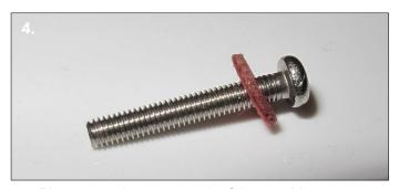
**4.** Place a washer over each of the two M2 screws.
