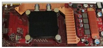
**4.** With the spring and metal washer in place, put a screw through the mounting plate and the hole on the card. Repeat this for each thumb screw.
