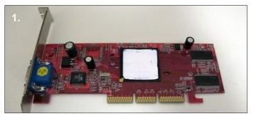
1. Remove the stock heatsink and clean the old thermal paste from the GPU core. Now apply new paste to the GPU.
