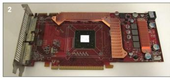
2. Apply new thermal paste to the GPU core.
