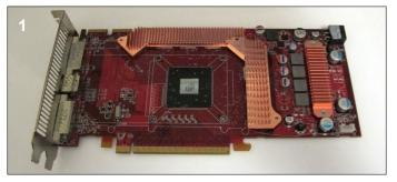
**1**. Remove the stock heatsink and clean the old thermal paste from the GPU core.
