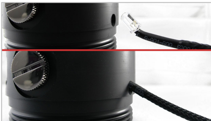
5. Slightly kink the LED wire and push the LED into the hole on the base of the reservoir. You might need to twist the LED slightly until it slots into place.
