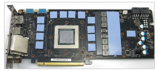
11. Remove the tape from both sides of the thermal pads. Place the blue and grey pads on the fifteen positions shown above and finally apply thermal paste to the GPU core. Place the waterblock on the card to line up the screw holes and then flip it over (make sure the thermal pads stay in place).
