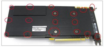
7. Now turn the card on its back and remove the 17 screws highlighted above.
