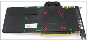
12. Place the waterblock on the card to line up the screw holes and then flip it over, making sure the thermal pads stay in place. First fit the M2.5 screws and washers (marked in red). Finally fit the original screws to attach it (marked in green). You should gradually tighten each screw to apply even pressure...
