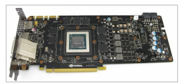
**9.** Clean the thermal paste from the GPU core and remove any residue left from the thermal pads.
