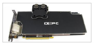
13. Do not over tighten the screws as this may bend the card and cause permanent damage. The card is now ready for use. When you first boot it is advisable to use software to check the core temperature. If the temperature is high you will need to remount the block.
