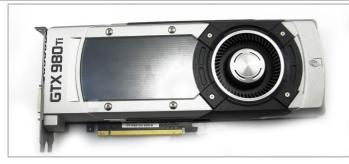
6. Before handing the card you should take precautions to avoid static damage. Remove the GTX 980 Ti card from the box ready for installation.
