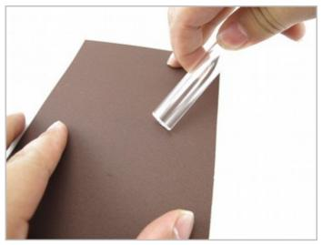
8. Use the sand paper to clean the chamfered edges of the tube. **Do not** sand the sides of the tube as this may stop the tube sealing in the fitting.
