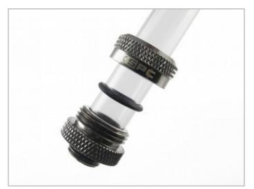
9. Place the compression fittings nut and o-ring over the PETG tube and push the chamfered end of the tube into the fitting. You will need to use some force to get the tubing past the two internal o-rings.
