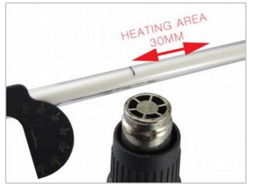
3. Slide the tube forward and heat it at the location of the mark, until it becomes soft. Make sure to rotate the tube to make sure heat is applied evenly. You can use a hair drier or heat gun for this. Don't get the heat gun too close to the tubing, or you will apply too much heat.
