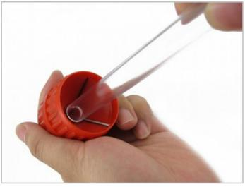
7. Use the chamfer tool to add an edge to each end of the cut tube. You must only rotate anti-clockwise. If you turn clockwise the blades will dig into the tube and give a poor finish.
