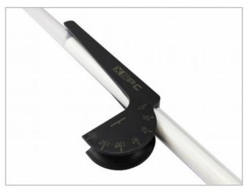
1. Soak the bending rubber in warm water before inserting it into the PETG tube. Now insert the PETG tube into the tool.
