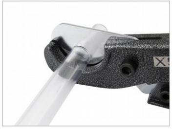
6. Remove the bending rubber and trim the edges of the PETG tubing to the correct length for your build. To remove the bending rubber, just twist and pull.
