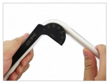
5. Bend the tube over the head of the tool until you get the desired angle. Hold it steady and allow the tube to cool before removing it from the tool.
