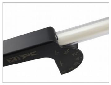
4. Slide the tube back into the tool, so that the mark lines up with the top of the tool.
