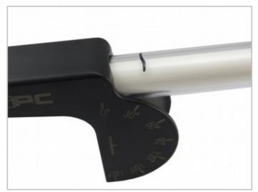
2. Make a mark at the intended bend location. When heating the tubing apply heat to the area in front of the mark. A 90° bend for example will take around 30mm of tube.
