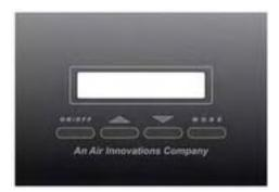
**Plug in the system.** Touch the on/off bottom on front panel. The display lights up to indicate power to the system. The system may not come on right away due to the timer built into the circuiting toprevent short-cycling. There is a 5-minute compressor/condenser fan time delay on initial start-up.
