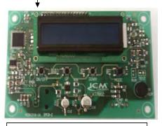
**Local User Interface**: Can be used with Main Control for adjusting settings, reading temp/humidity, and reading fault codes at the unit.
