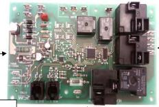
Two way communications: local user interface reports settings back to main control, main control energizes outputs and reports alarms and temp/humidity readings to local user interface.
