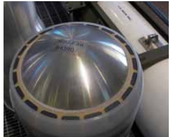
Thermonuclear physics package—plutonium pit and highly enriched uranium secondary—of a W80 warhead.
