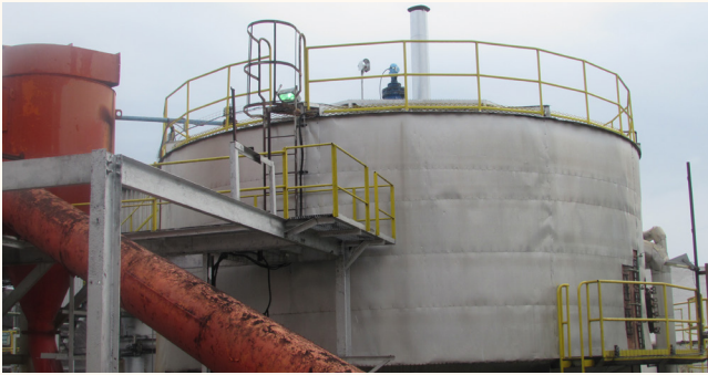
Specially Designed Sugar Research Institute Clarifier
