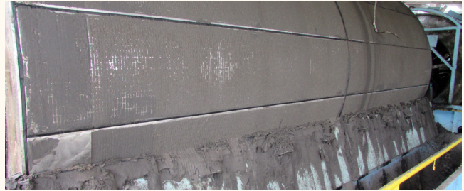
Mud Filters used to remove Settled Mud
