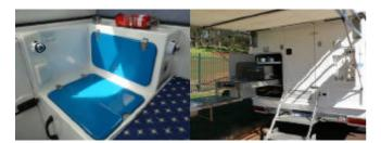
**A16.** If the external kitchen is NOT fitted to the unit, then the space between the utensils' storage compartment and the floor can be used as a general storage area. If the external kitchen is fitted, it occupies the top part of this area and there is a storage area running underneath the external kitchen right through to the gas storage compartment at the front of the slide-on. (Photo above)
