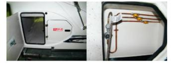
**A12.** The beds are hinged at the front so that they can lie horizontal for sleeping. A gas strut passes through the bottom and pushes against the lid. When the lid is unlatched, it and the mattress are pushed up against the roof allowing access, at a convenient height, to the contents of the "suitcase". When the two halves of the bed are locked together, the gas struts enable the whole bed including its contents and mattress to be raised effortlessly to the roof.
