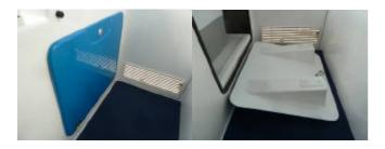
**D5.** The top compartment of the toilet unit contains water for flushing and the bottom part has a very effective seal to prevent any odours escaping when the toilet is not being used. The toilet is located in an area where the refrigerator fan blows air around it and out through a vent to the exterior of the van when the Slide-on roof is raised.
