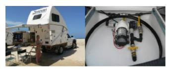
**A29.** Unless there is a request by a customer to do otherwise, two 55 L water tanks will be mounted so that one sits on top of the other. That arrangement leaves plenty of room for extra water containers to be placed in front of the tanks for those occasions when extra water would be required. If an air-conditioner is to be fitted to the unit, then the two tanks need to be positioned beside each other so the air-conditioner can be fitted above them.
