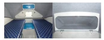
**A24.** The front window is normally fitted so that the blind pulls up from the bottom. This allows for more privacy and also prevents splashes of rain coming into the unit. The screen and blind can be moved to the desired position and the double glazed window can be hinged out and locked in a number of positions.
