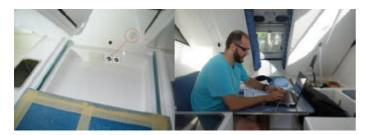
**A22.** LED lights use a lot less electrical energy than conventional lights and they produce much less heat and so will not cause a burn or a fire as other types of bulbs might do. All the lights in the XS Innovan are LED lights. There are two lights located on the outside of the back wall under the awning, two in the storage compartment and in the interior of the unit, there are six adjustable reading and work lights and one strip light.
