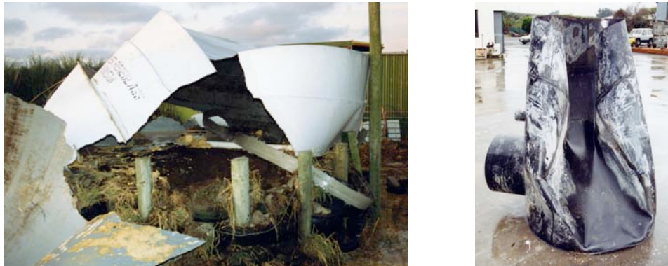
Fig 8: Fibreglass tank failure is sudden and dramatic (left) compared to plastic failure (right)
