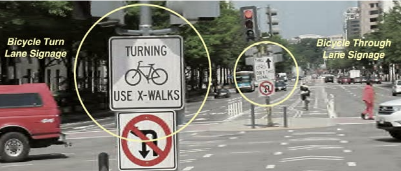
Signage for turning bicycles
