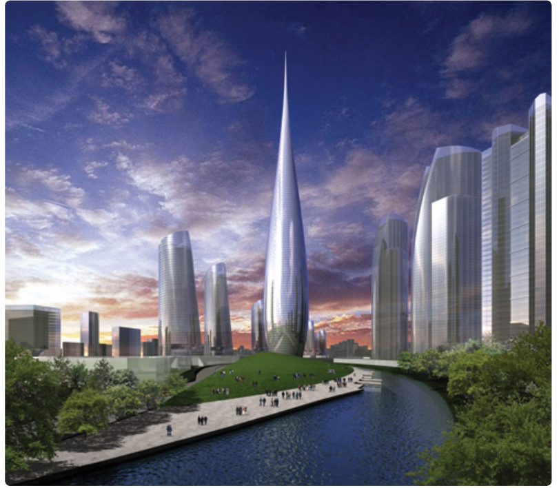
SOM, Yongsan office tower competition, Seoul, Korea, 2009 The structurally efficient teardrop shape for the building was revealed through the use of a genetic algorithm.
