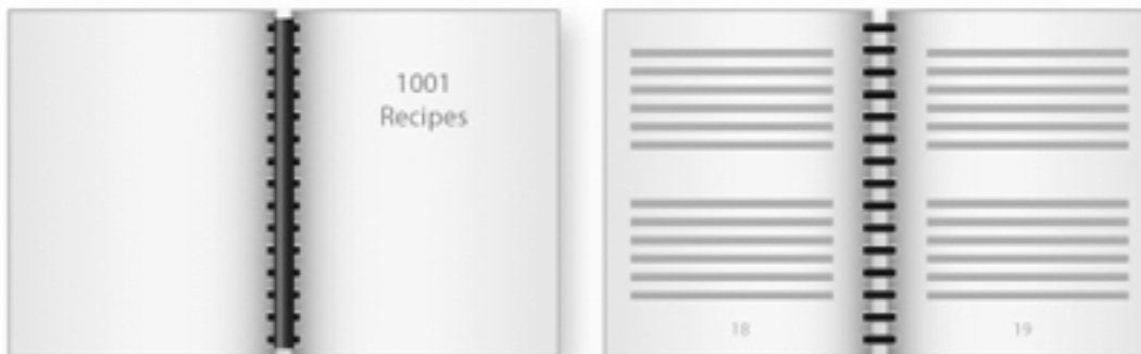
Figure 4: Comb binding allows books to be opened flat but makes a printed spine
