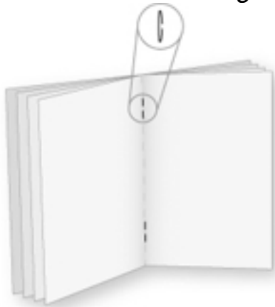
Figure 1: In saddle stitching, wire is fed from a roll, bent into shape, the legs are forced through the signatures and then bent into the staple shape.
