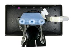
The QuadStick has a joystick, four sip & puff sensors, a lip position sensor, and a push switch connected to a 32-bit ARM processor that converts the sensor inputs into USB and Bluetooth signals for PC's & Game consoles.
