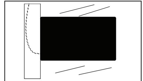
Adhere the backing label to the opposite side of the glass to block the back of the Surface Mount and iPad.
