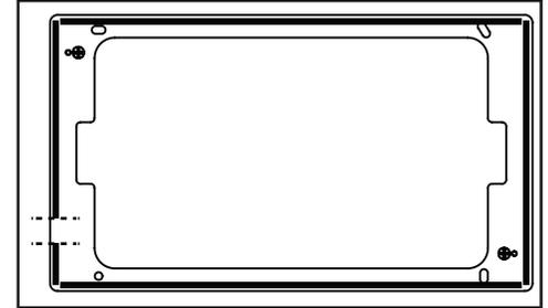
Cut a piece of the adhesive strip where the lightning cable will route behind Surface Mount.
