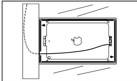
Connect the iPad and place it in the bezel. (See Surface Mount Instructions) Attach the bezel to the bracket. Adhere the Surface Mount to the glass close to the channel.
