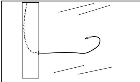
Drill a 3/8" small hole and route the lightning cable down the aluminum channel and out the hole. Make sure there is enough length.
