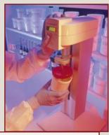
The Electronic Mortar & Pestle (EMP) creates pharmaceutically elegant ointments, creams, gels and suspensions. Components are weighed, mixed and dispensed in the same jar, eliminating compounding time, clean-up and waste.
