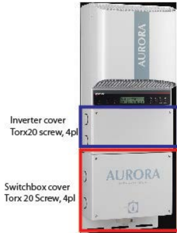
Figure 2:02- Location of Front Access Panels
