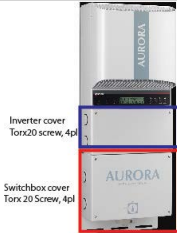
Figure 4:02: Location of Front Access Panels
