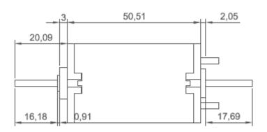
2) Motor and worm double reduction gearbox (14:1, 25:1 or 33:1 ratios) unit with 3/16" axle
