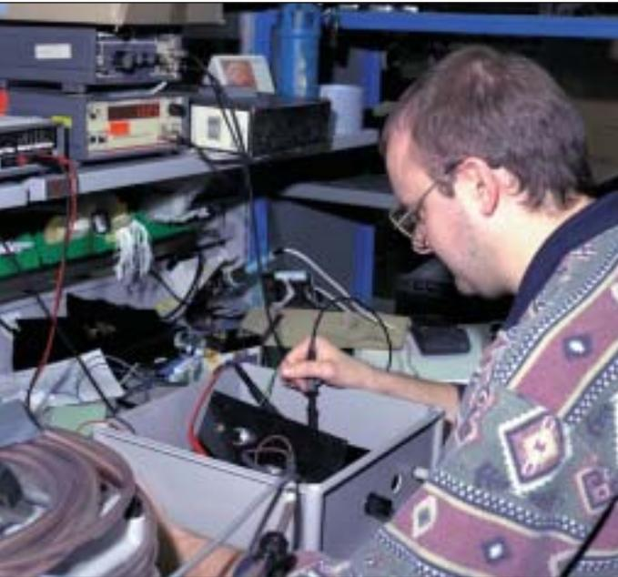
should be tested at least annually using an RCD tester which will check the tripping current and the speed of operation.
