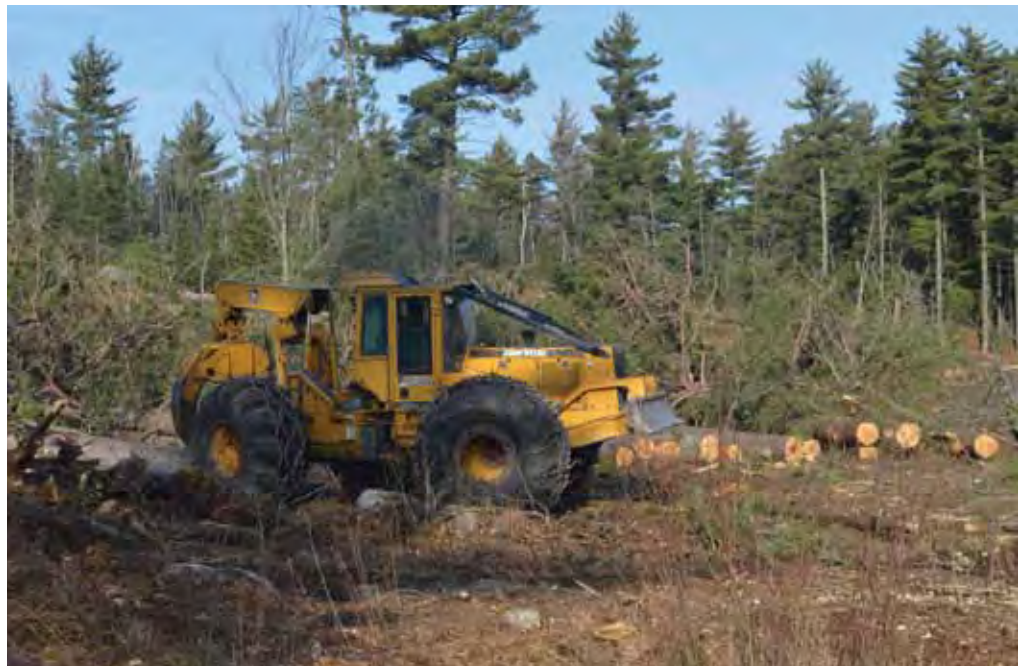
Because the Rolle crew skids the wood to the landing after it has been delimited, he feels he realizes a significant saving in fuel costs. The company utilizes this John Deere 648G skidder, as well as a Deere 748H.
