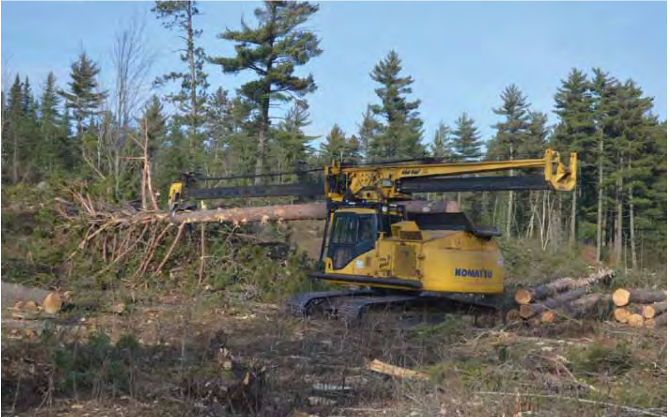
Rolle's Komatsu delimber with a Pro Pac boom limbs the wood throughout the sale rather than at the landing. Rolle also has a John Deere with a Denharco boom.
