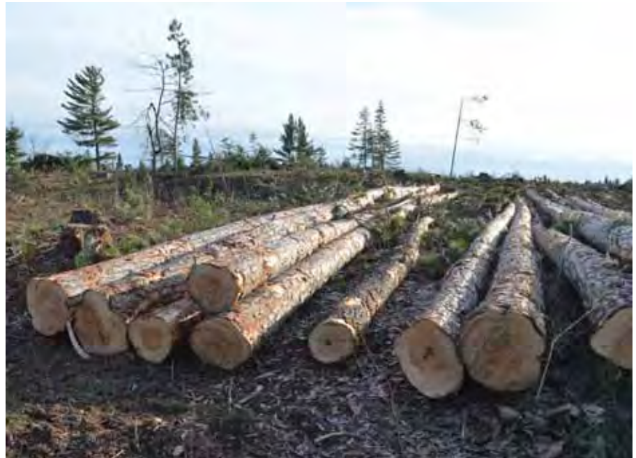
Once the timber is delimbed, it’s lined up with the butts facing the same way for easier skidding and sorting.
