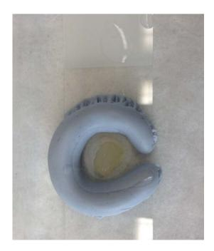
22. With the lipped side facing up, firmly press a Willco dish down onto the adhesive until it just comes into contact with the sample. Using a pipette, add more PROTOS to the gaps between adhesive until the imaging chamber is filled.
