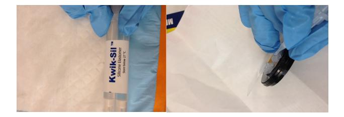
24. Cover this construction with aluminum foil and store it away safely to cure. After about 20 minutes, the sample is ready for imaging.
