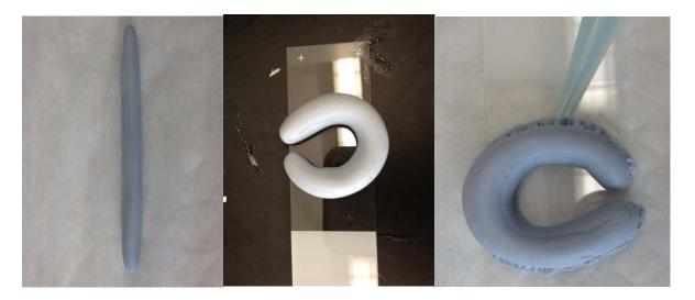
21. Carefully place the sample in between the Blu-Tack pieces and add about 20  $\mu$ L of PROTOS to the sample.
