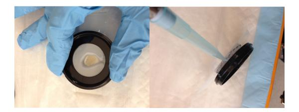
23. KWIK-SIL is an adhesive that cures rapidly. Carefully add it to the gaps between the Blu-Tack to build a wall and seal in the sample. Take care not to introduce any bubbles, and make sure the chamber is completely filled with PROTOS.
