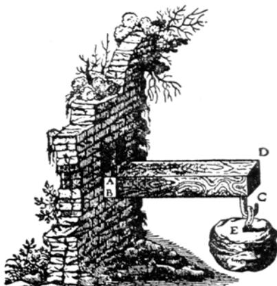
Cantilever beam according to Galileo (1638) and evolution of the “hypothesis” for the stress distribution at AB
