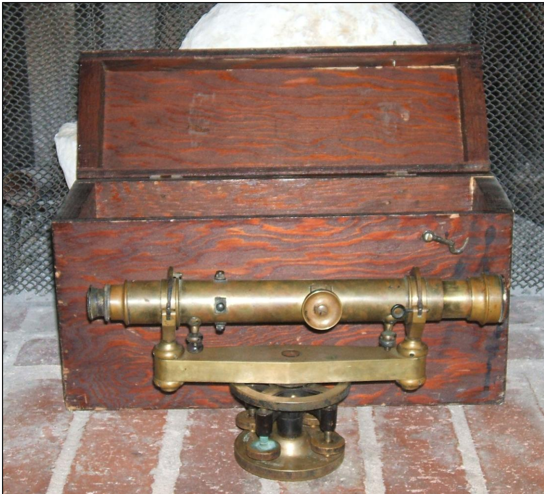
Figure 2. Example of Surveyor's Level from AGS member John Mikels. This level was likely manufactured in the late 1800s to early 1900s.
