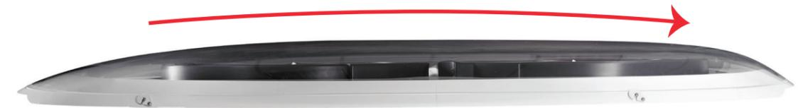
Using Computational Fluid Dynamics (CFD) analysis, the longer – and lower profile – 2Ku radome was modeled against a radome for a traditional gimbaled antenna on an A320 airframe. The result was 31.7 lbs. (14.4 kg) of drag for the traditional gimbaled antenna radome vs. 6 lbs (2.7 kg) for the 2Ku radome.
