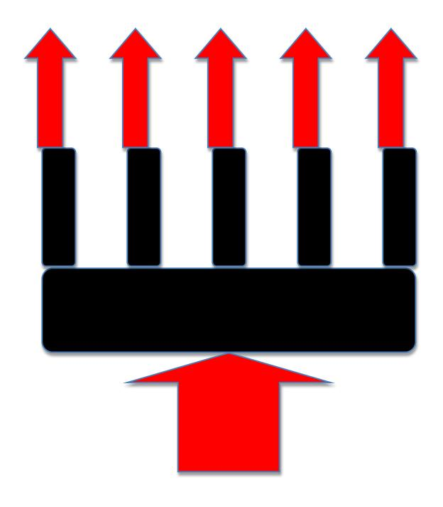
**Erosion Control Guidelines: Dewatering Use manifold to reduce velocity and volume**
