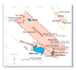
Understanding this geometry is a key component to designing an optimum open pit shell shape to capture a maximum of ore grade material. The current exploration programme will drill within and adjacent to the known mineralisation to boost the Mineral Resource while also targeting known high grade zones that might add to early higher grade mineralisation.
