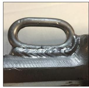
In the case of the Leatherhead Tools halligan, the shoulders come pretty square right from the factory. The only snag in their fork set-up is actually the shaft of the bar, not the fork itself.
