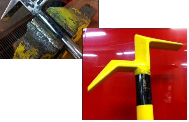
To our Pigs, we apply two coats of Rustoleum Rust Inhibitor (clear-coat), or just plain Rustoleum clear-coat spray-paint. Every few months, or whenever it needs it, we strip it off with a wire-wheel and re-apply.
