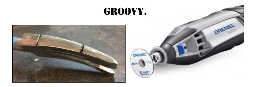
A Dremel Tool with a metal-cutting blade attached is also a good plan for marking the fork and adz with gap-lines and set-line. A little finer than using an angle-grinder.
