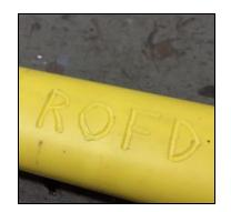
With a smooth and steady hand, write your letters into the handle. Take care to just melt the surface plastic. Once cool, fill in the grooves of the lettering with a sharpie or a paint marker.
