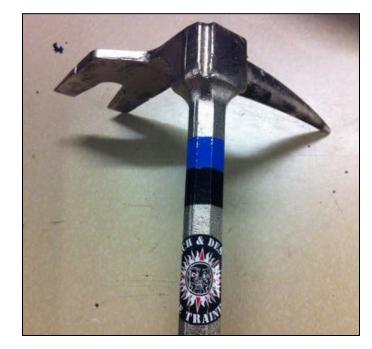
4 – Consider using a clear-coat spray-paint as a second coat. This will lessen chipping.
