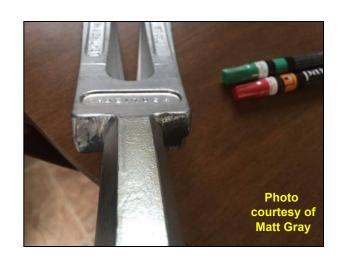
The 3-piece version of the Zico Quic-Bar also has a hexagonal shaft, making any kind of shoulder-striking potentially more difficult.
