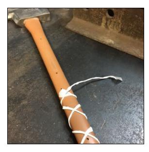
Again, make the intersections of the downward spiral and the upward spiral neat and uniform up the handle. You can adjust them slightly by moving the sticky-string that makes the upward spiral.
