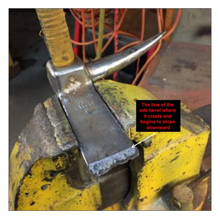
Next, use a ruler or other straight-edge to mark a straight line along the crest of the adz bevel, where it starts to angle downward.
