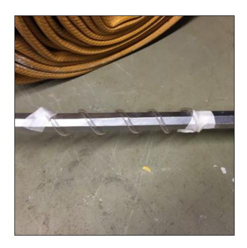
If you're using hockey tape or med tape to make a twisted-tape under-material, cut one section of tape, 30" long. Then stick one end to something that's not going to move, and hold the other end in your left hand. Pull the piece of tape taut.
