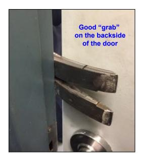
After gapping an <u>outward-swinging door</u>, the angle of the tool should be adjusted slightly and driven in further until the set line is between <u>the front-edge of the door and the rear edge of the door</u>.
