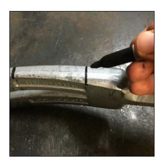
First, measure each side of the fork, 1-3/4" down from the fork-tip. Mark the side of the fork with a sharpie or soapstone marker.
