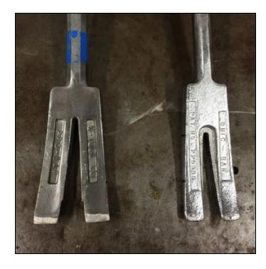
The depth of the opening in the "crotch" can vary from one manufacturer to another. This is something to bear in mind when filing or grinding set lines into the fork. You may want to take a quick second to measure yours before marking it.....uh, the one on the *halligan*.
