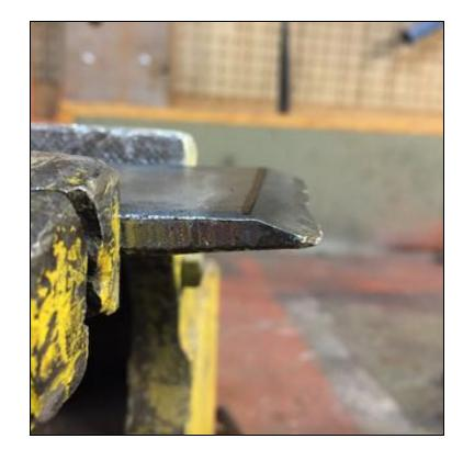
Now that you have the under-side ramp gone for good, flip the tool over in the vise so that you can work on the top-side to create a more useful bevel.
