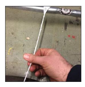
Mark the shaft where you intend the tape-wrap to start and stop.
