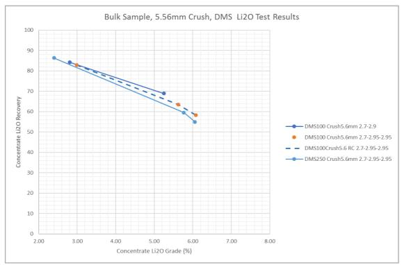
Figure 5: DMS100 and DMS200 - Grade Recovery test results
