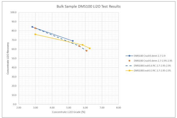
Figure 4: Dense Media Separation 100 – Grade Recovery test results
