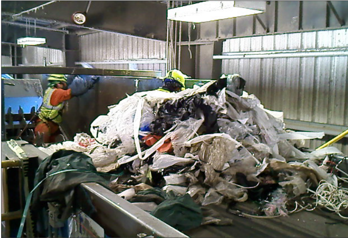
Photo 12 - Plastic Bags and Film Removed from Equipment at the Davis Street Transfer Center in San Leandro
