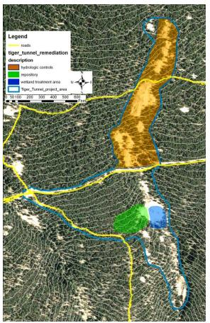
The Tiger Mine Restoration Project involves removing a large mine waste pile, constructing a repository for the waste, installing hydrologic controls, and constructing a sulfate reducing bioreactor (a.k.a "wetland treatment system").
