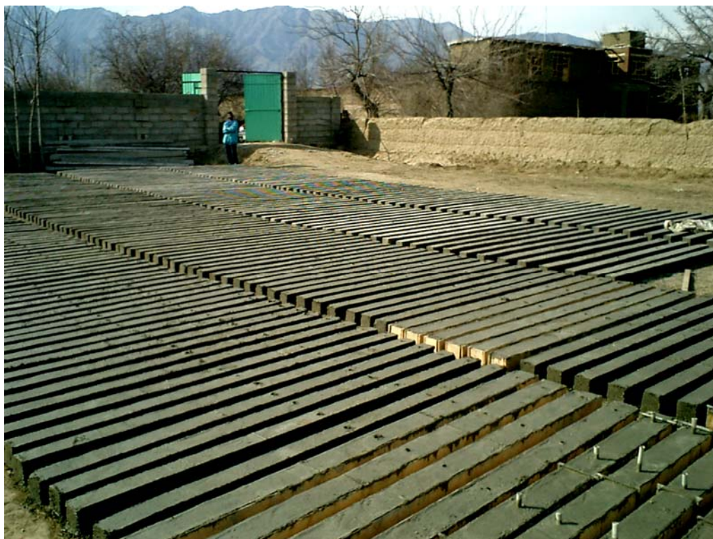
Concrete trellis posts under construction near Bagram, February 2006.
