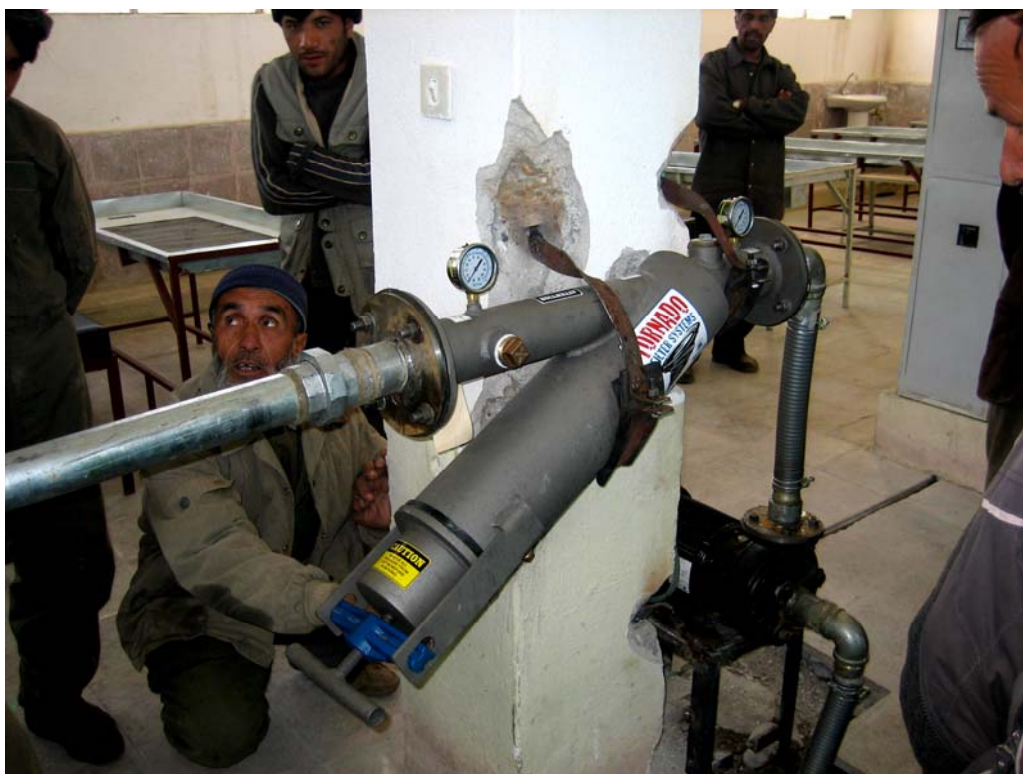
Water pump and water filter for raisin processing line installed at Charikar plant in participation with ROP, November 2005.
