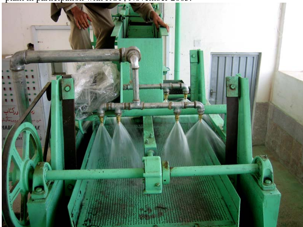
Spray nozzles on raisin processing line installed at Charikar plant in participation with ROP, November 2005.
