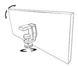
The included mounting clamp attaches to the back of the *TC-Display* and can be used as an adjustable tilt stand.
