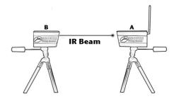
Turn on *TCi-PhotoGate B* by holding down the *On/Off* button until the desired power level is selected.\* The blinking green light indicates the unit is on. *TCi-PhotoGate B* emits an infrared (IR) light beam that is detected by *A*.
