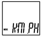
KPH/MPH mode calculates kilometers per hour and miles per hour.
