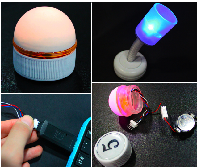
Figure 3: a)Ping; b)Wax-E; c)Ping is open so we can see battery and connector; d)USB connection to the PC
