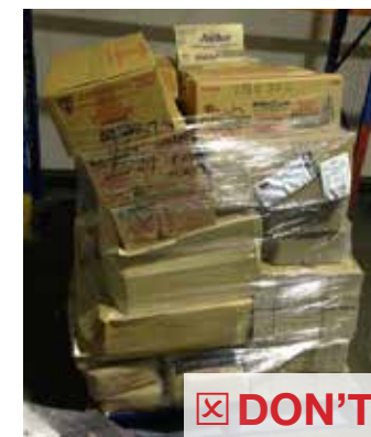
No solid base foundation to build a pallet. Cartons on top were heavier than bottom layers
