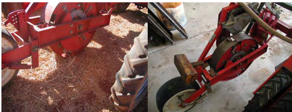
A planter with lengthened cups for direct-seeding rockmelons into mulch (left) and a seeder used for planting zucchini seed directly into cereal residue
