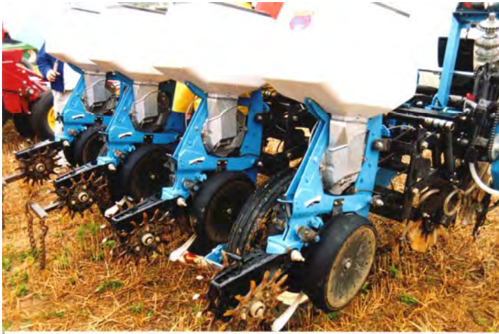
A no-till seeder produced by Monosem TM . Note: coulter disc to slice through surface mulch.
