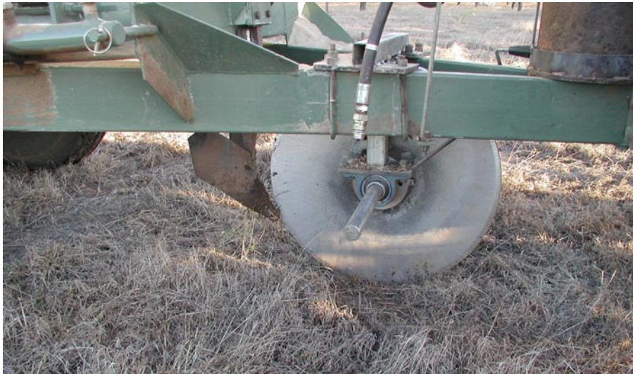
Figure 3.2.2: Cutting disc and boot assembly.
