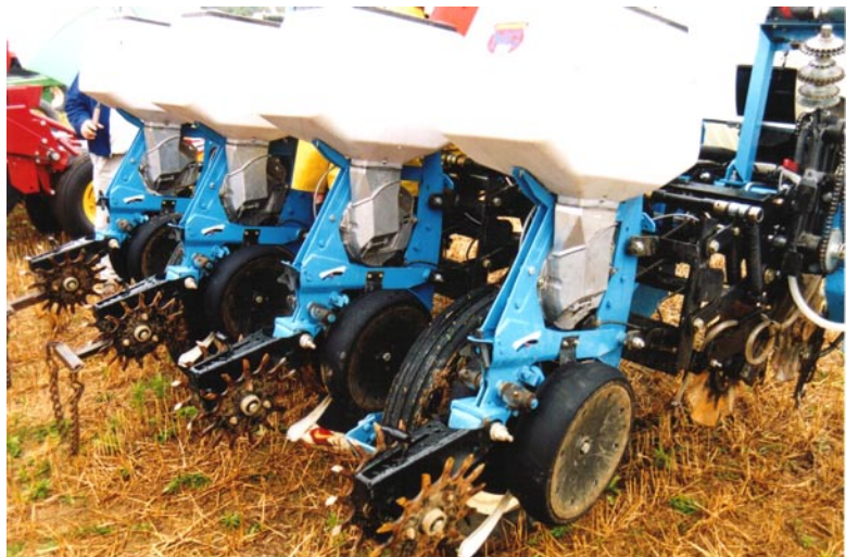
A no-till seeder produced by Monosem™. Note: coulter disc to slice through surface mulch.
