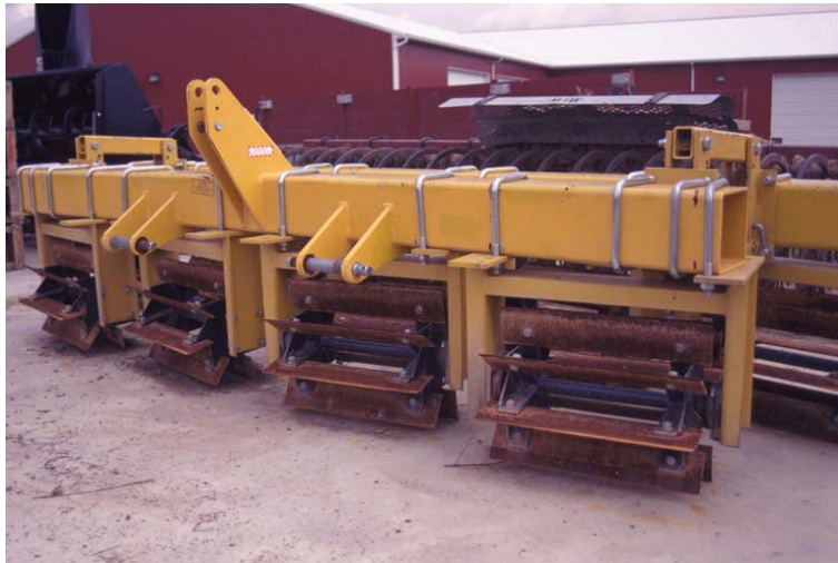
Corn Stalk Chopper used in the USA to kill cover crops in preparation for planting
