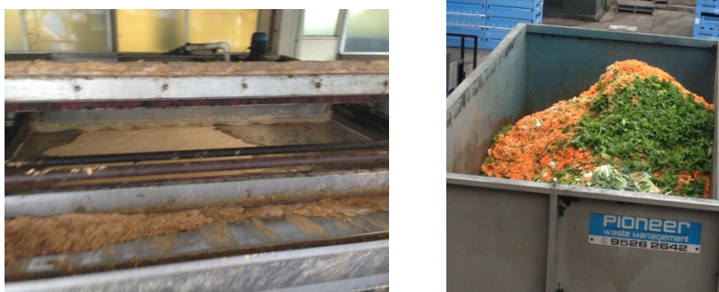
Figure 22 - Vegetable 'sludge' made from ground, flocculated vegetable waste.
