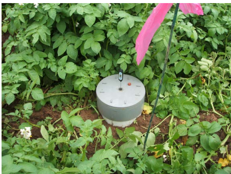
Image 4: Illustration of a manual static gas chamber in a potato crop at Grech Farms, Theresa Park. Note the septum on the lid and thermometer used to measure internal chamber temperature.
