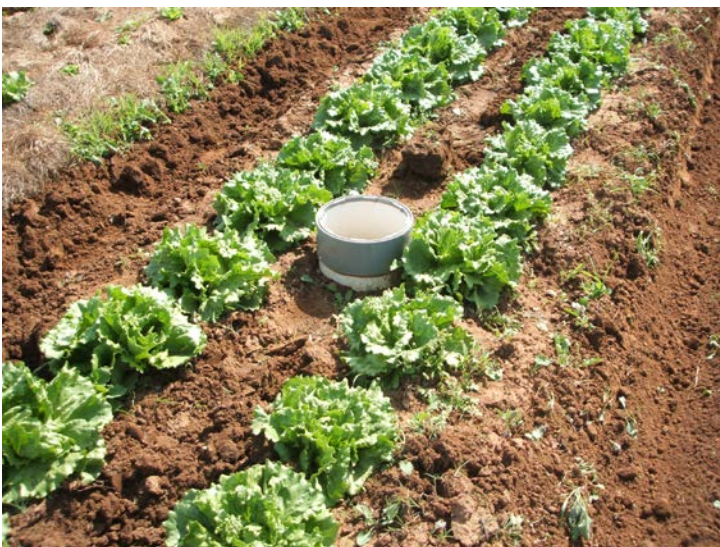
Image 6: Example of the placement of gas sampling chambers in the inter-row area of crops.
