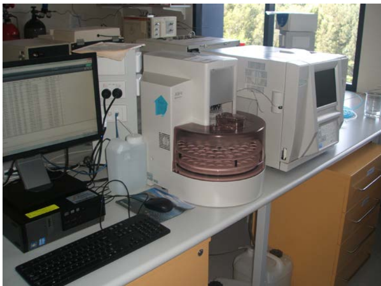
Image 8: Shimadzu total organic carbon analyser and total nitrogen measuring unit used to determine soil microbial carbon and nitrogen.
