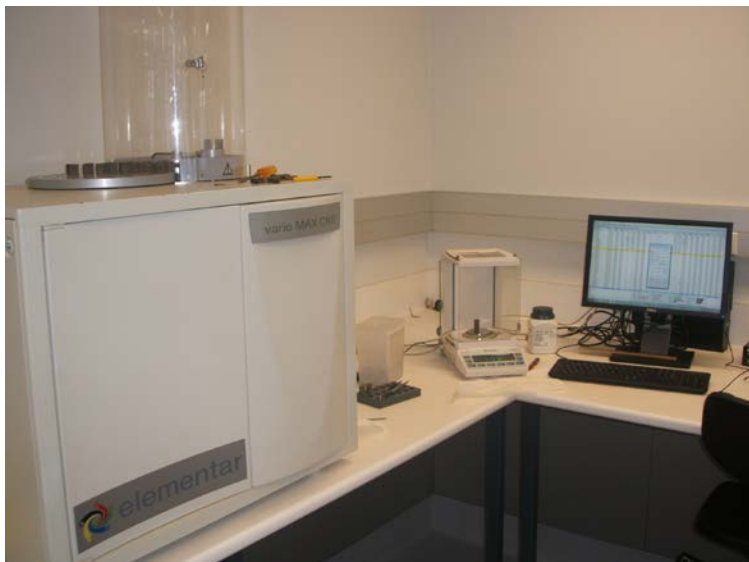
Image 9: Elementar carbon and nitrogen analyser used to determine total soil carbon and nitrogen.
