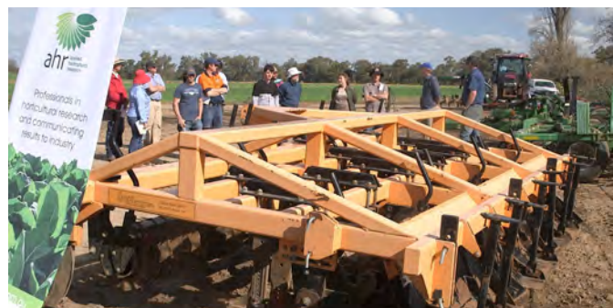
Implement to incorporate crop and cover crop residues with minimal soil disturbance.
