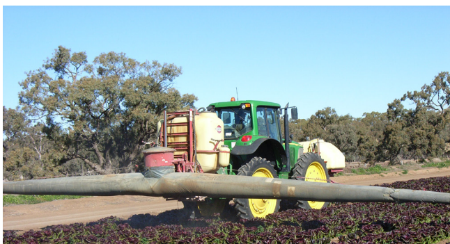
Air assisted boom in lettuce crop
