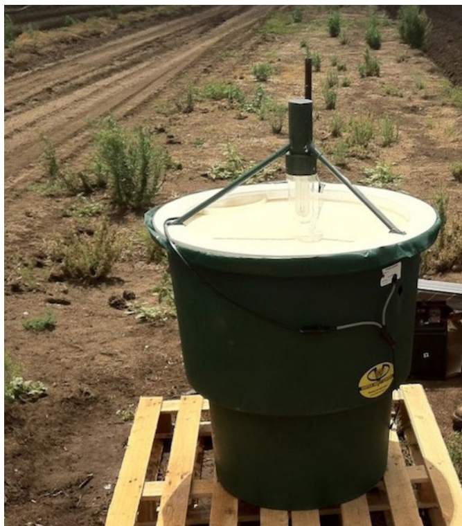
Figure 4. Vortex light trap and impact of the light trap on moth numbers in a baby leaf spinach crop in SE Qld.
