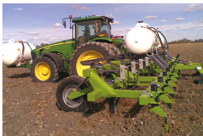
Figure 2 - Anhydrous ammonia 'BiG N' application equipment using tines. Photo courtesy of Incitec-Pivot Fertiliser.
