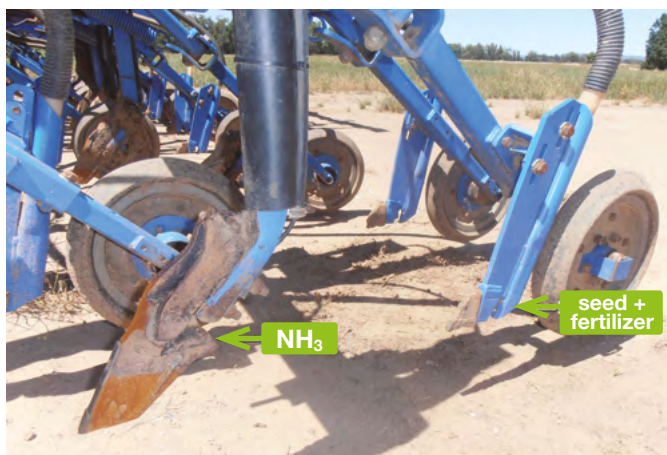
Figure 5 - Side view of the knife point for anhydrous ammonia and granular seed/ fertiliser on the application equipment on the commercial vegetable farm in Cowra, NSW.
