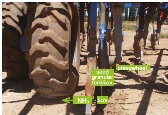
Figure 6 - Front view of the knife point for anhydrous ammonia and granular seed/ fertiliser on the application equipment on the commercial vegetable farm in Cowra, NSW.
