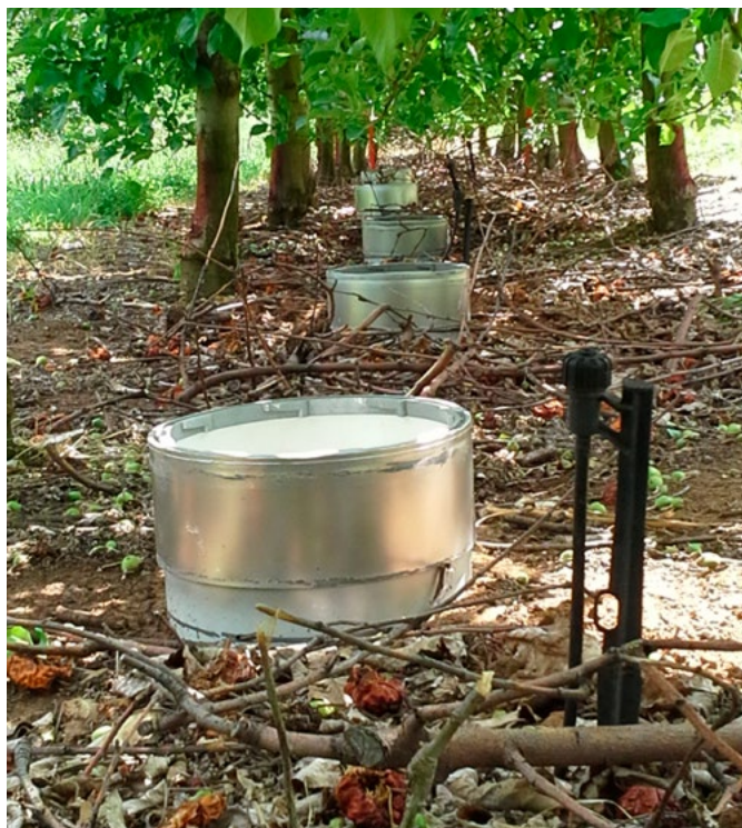
Chambers used to measure nitrous oxide emissions from the soil in apple/cherry orchards.
