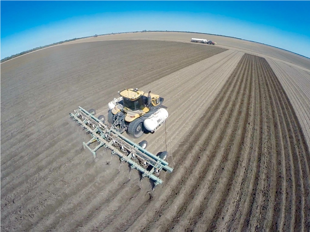
Figure 5. Anhydrous ammonia Big N being applied into rows. Photo courtesy of Incitec Pivot Fertilisers.
