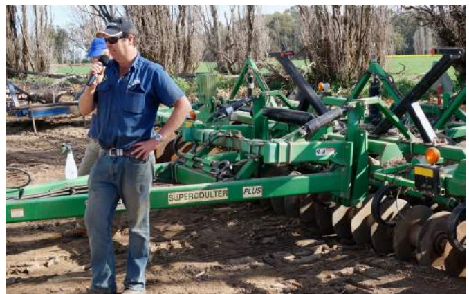
James Fagan with planter designed to sow cover crops through crop residues without cultivation.
