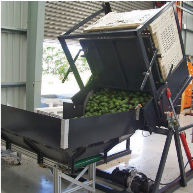
Dry bin tippers should include a cover, so that fruit is fed out gradually. Wet bin tips avoid impact damage, but the water must contain a sanitiser
