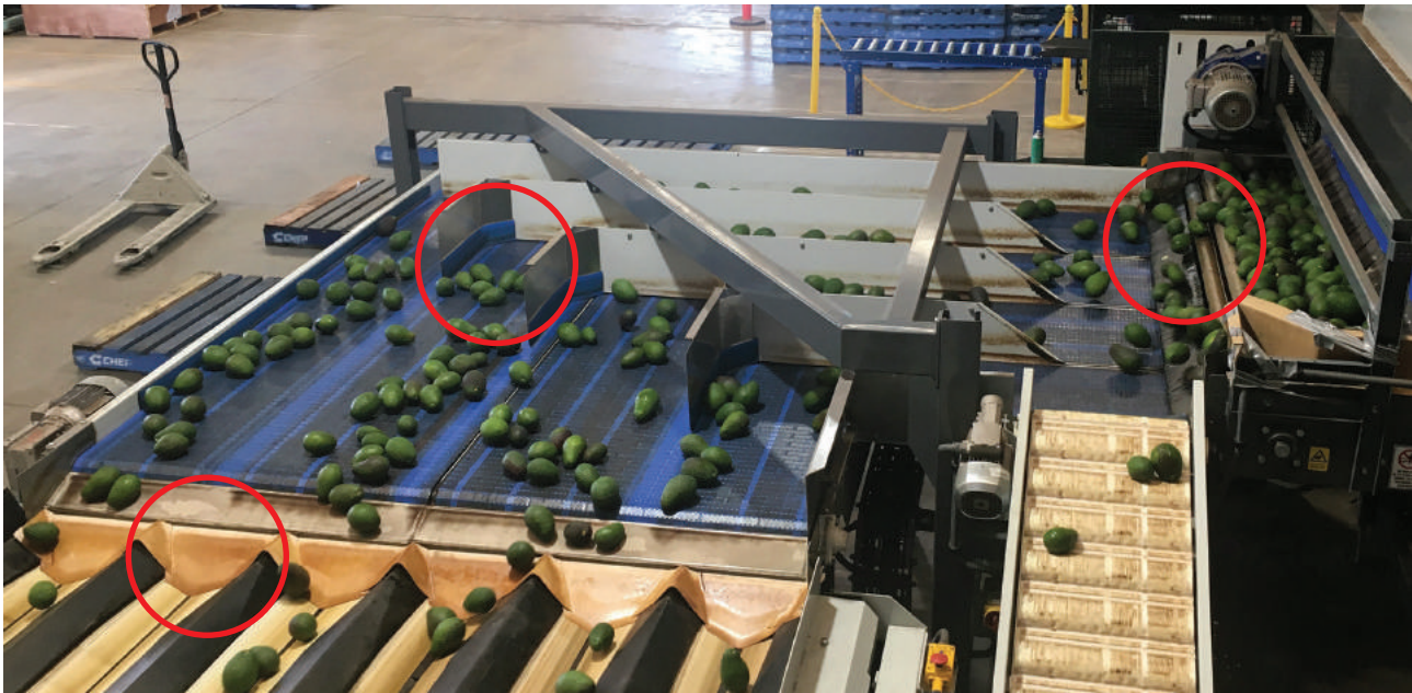
Packing lines should have baffles and padding to minimise drops (circled in red). Speed should be adjusted so that fruit do not accumulate and knock against each other.
