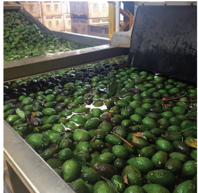
Dry bin tippers should include a cover, so that fruit is fed out gradually. Wet bin tips avoid impact damage, but the water must contain a sanitiser
