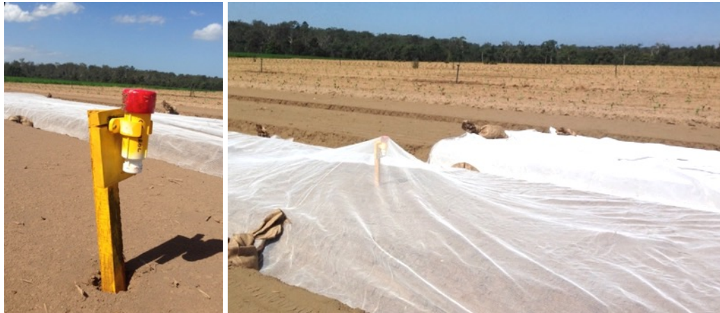
Figure 23. Hobo data logger installed in the open, uncovered area of the bed and under a floating row cover
