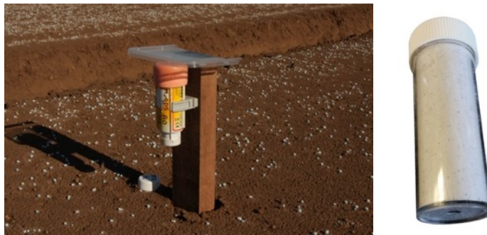
Figure 43. Installation of temperature loggers: A Hobo UX100 was used to monitor air temperature and RH, while an i-button buried inside a small tube monitored soil temperature (only lid visible at left, i-button at base of tube at right).
